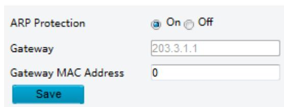
2. Select the check box to enable the ARP binding function and set the gateway MAC address.
