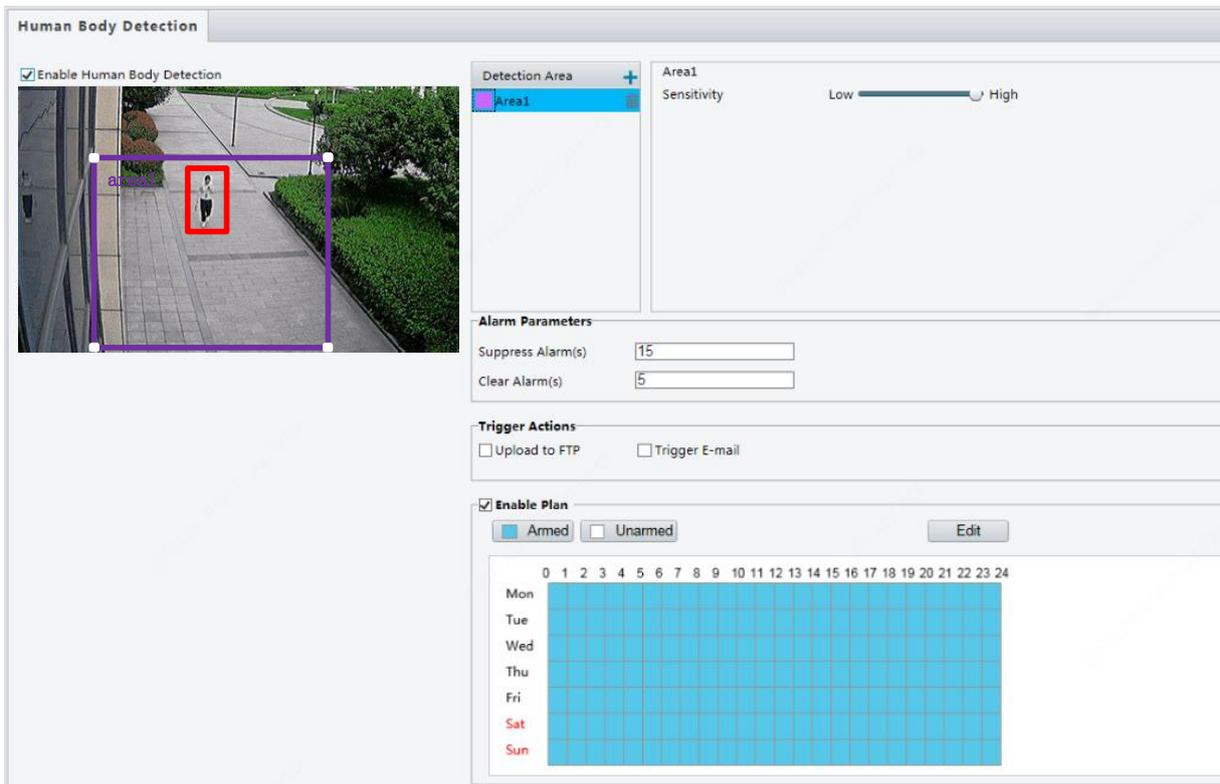
2. Select the checkbox of **Enable Human Body Detection**.
