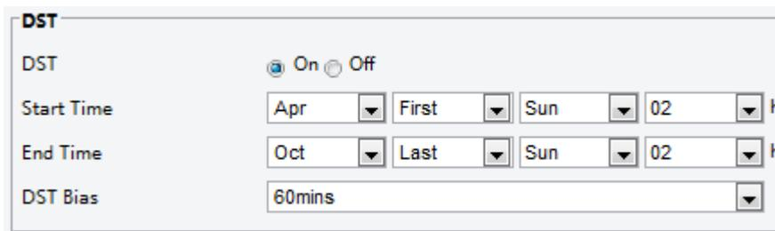
The screenshot shows the 'DST' configuration page. It features a 'DST' section with a radio button set to 'On'. Below this are two rows for 'Start Time' and 'End Time', each with four dropdown menus for month, day type, day of week, and hour. The 'Start Time' is set to 'Apr', 'First', 'Sun', '02' h. The 'End Time' is set to 'Oct', 'Last', 'Sun', '02' h. A 'DST Bias' dropdown menu is set to '60mins'.
