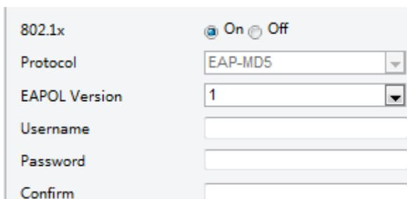
The image shows a configuration form for 802.1x. It includes the following fields: '802.1x' with 'On' selected, 'Protocol' set to 'EAP-MD5', 'EAPOL Version' set to '1', and three empty text boxes for 'Username', 'Password', and 'Confirm'.
