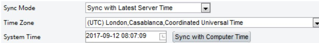
The screenshot shows the 'Time' configuration page. It features three main sections: 'Sync Mode' with a dropdown menu set to 'Sync with Latest Server Time'; 'Time Zone' with a dropdown menu set to '(UTC) London,Casablanca,Coordinated Universal Time'; and 'System Time' with a text input field containing '2017-09-12 08:07:09' and a 'Sync with Computer Time' button.
