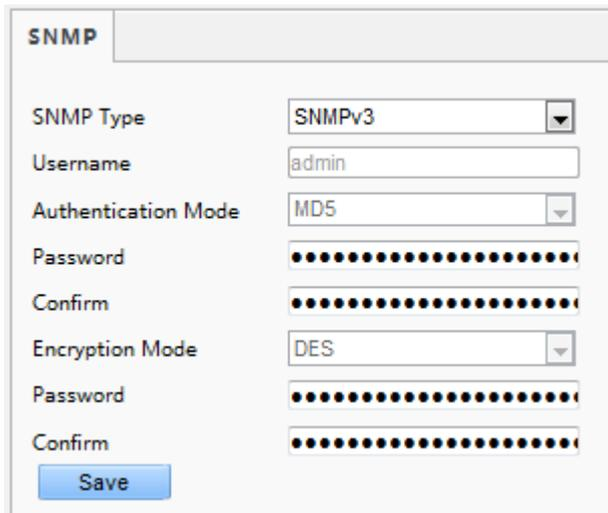
The image shows a configuration form for SNMPv3. It includes the following fields: 'SNMP Type' set to 'SNMPv3', 'Username' set to 'admin', 'Authentication Mode' set to 'MD5', 'Password' (masked with dots), 'Confirm' (masked with dots), 'Encryption Mode' set to 'DES', and another 'Password' (masked with dots) and 'Confirm' (masked with dots) for encryption. A 'Save' button is at the bottom.
