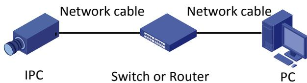
Use Shielded Twisted Pair (STP) cables to connect the network interfaces of the camera and the switch or router.
