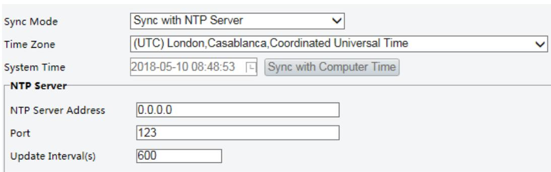
The screenshot shows the 'Time' configuration page with NTP server settings. It includes 'Sync Mode' set to 'Sync with NTP Server', 'Time Zone' set to '(UTC) London,Casablanca,Coordinated Universal Time', and 'System Time' set to '2018-05-10 08:48:53'. Below these is an 'NTP Server' section with three input fields: 'NTP Server Address' (0.0.0.0), 'Port' (123), and 'Update Interval(s)' (600). A 'Sync with Computer Time' button is also present.
