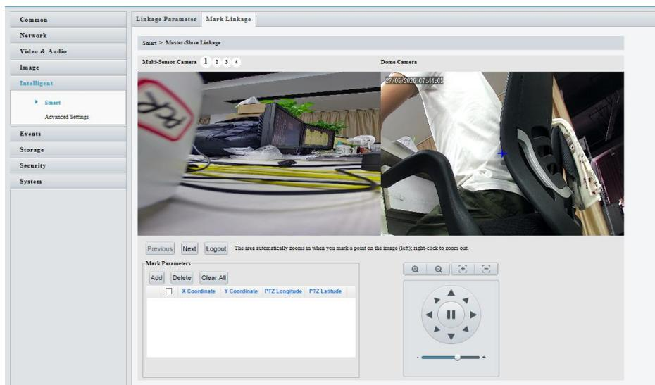
10. Marking steps on a single scene: Click **Add**, click on the left master camera image. A small white frame appears at your clicking, and the area automatically zooms in (as shown below). Adjust the position of the marking point on the enlarged area. Right click to return to original image and select again. Click **OK** to confirm current marking point.
