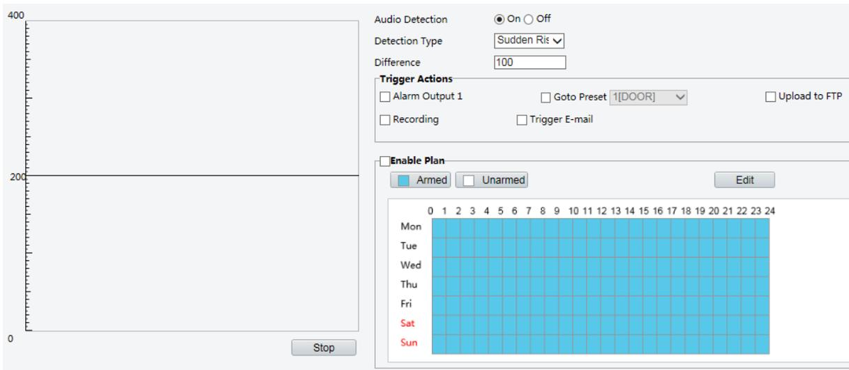
2. Select **Enable** for **Audio Detection**, select a detection type and set the difference or threshold. To disable audio detection, clear the **Enable** check box.
